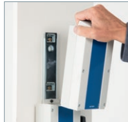
Spare battery on the wall charging station
