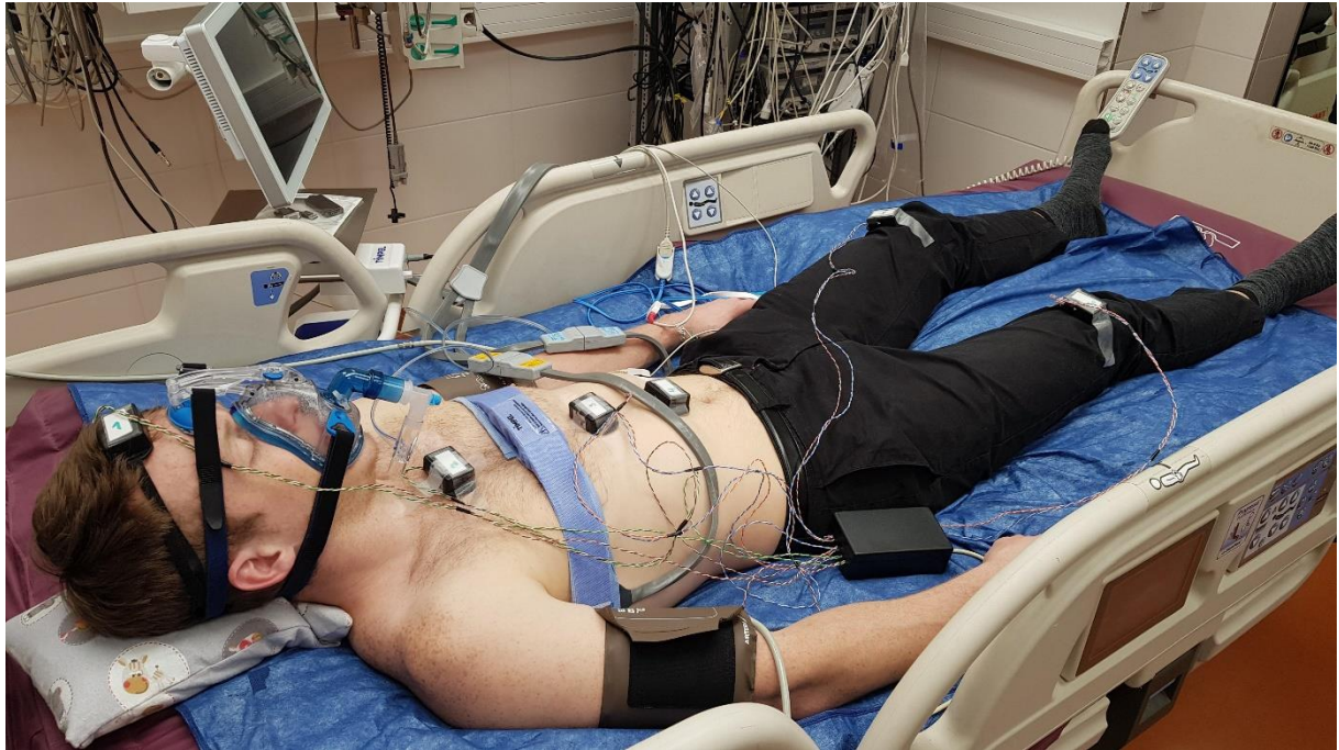
Figure 2: Body and sensors setup on the Hill Rom bed
